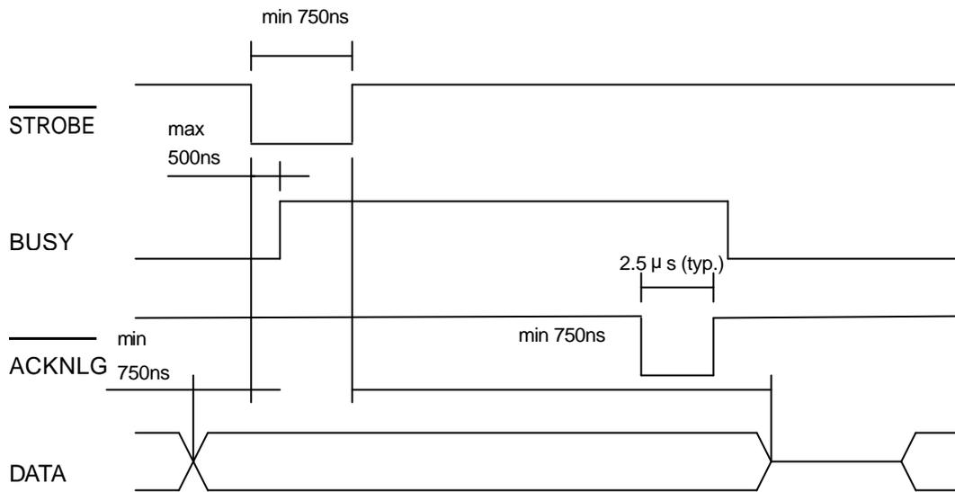
ACKNLG "LOW" indicates that the printer has received data.
