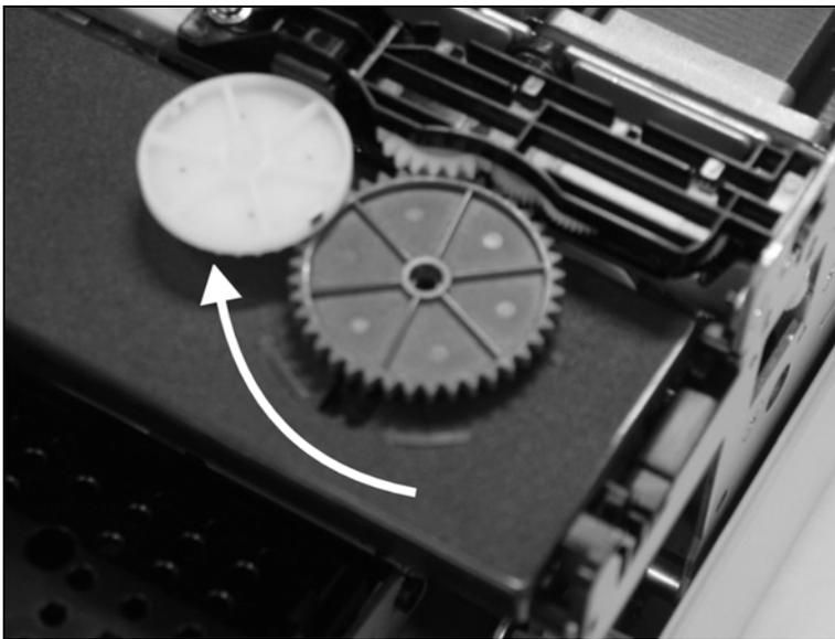
Ensure that the ribbon material is moving correctly by turning the tension gear in the direction of the arrow.
