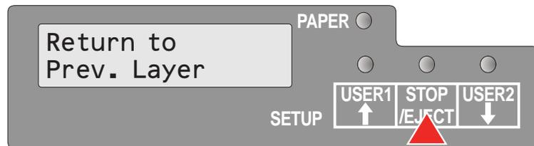
Press the **STOP/EJECT** key.
