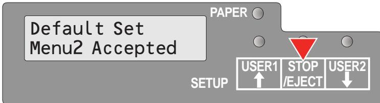
If pressed after you have changed a parameter item the new value is confirmed. The LCD displays the message **Accepted** after the parameter item is changed.
