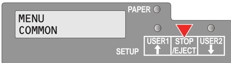
The **STOP/EJECT key** is used to select the next menu level (e.g. **MENU USER > Default Set User 1**), to open a parameter item for changing and to confirm changed parameter items.
