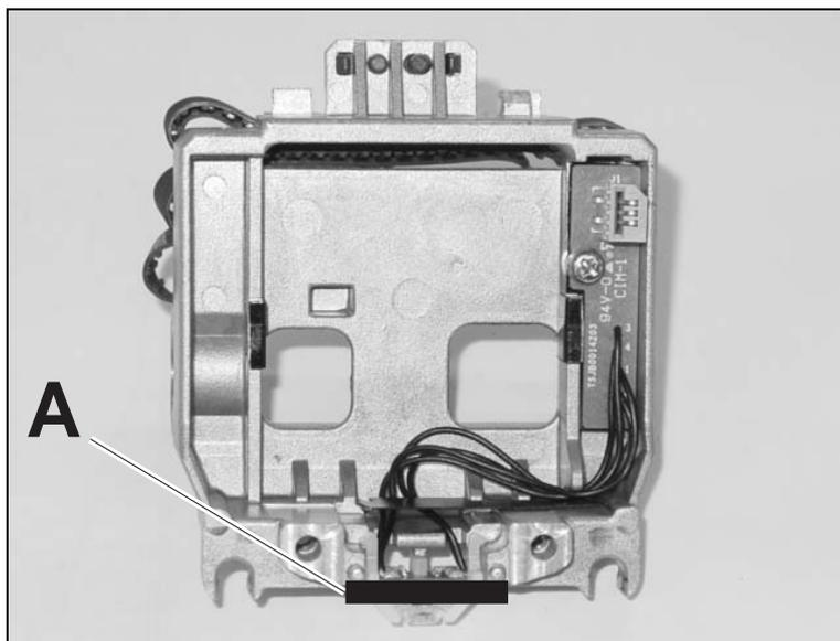
Ease the new print head down into the mounting.
