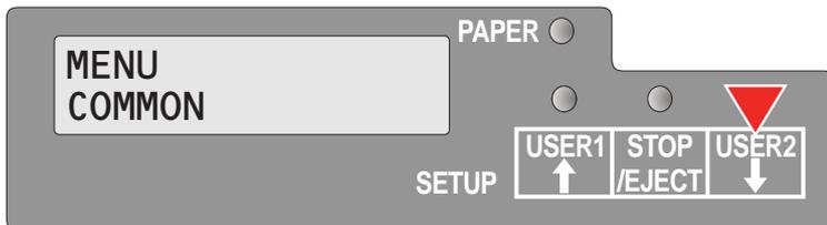
The **USER2 key** is used to go to the next parameter group or next parameter on the same menu level (symbolized by an arrow pointing downwards).
