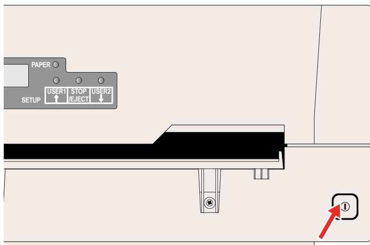
Switch the printer off and on again in order to set the printer in the normal operating mode.
