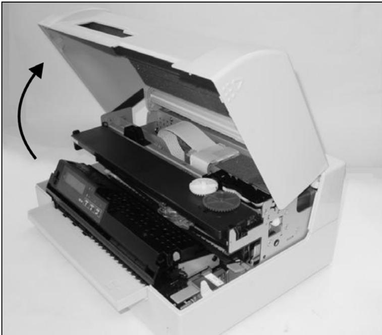
Open the top cover by grasping it at the right and left-hand side and swing it upward until it clicks into position.
