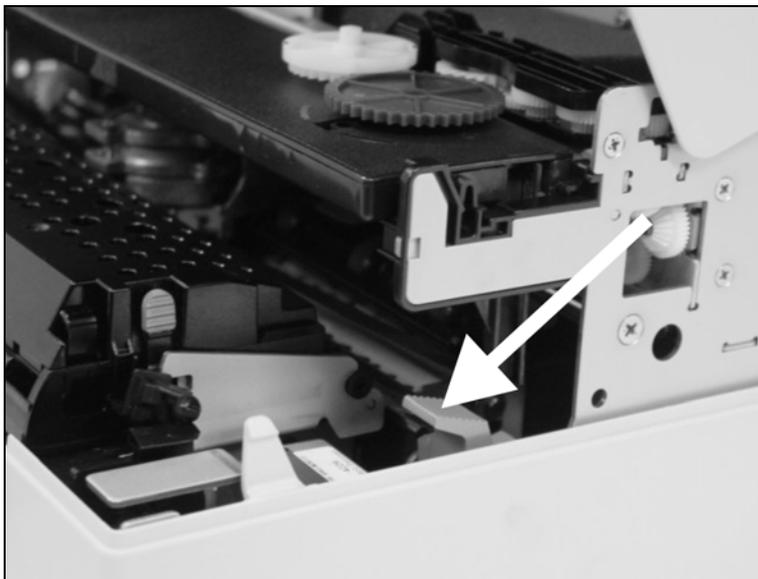
Press the green release lever for the printing mechanism. This swings the printing mechanism backwards.
