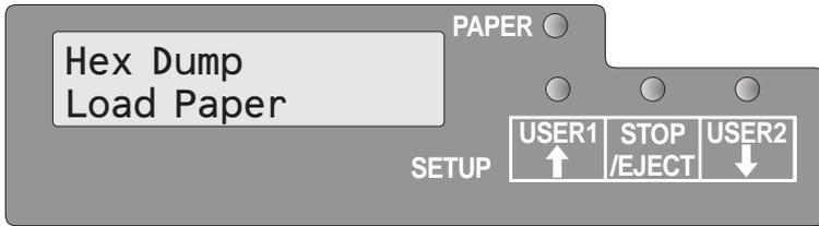
If the printer receives data when there is no paper in the printer, the message will be changed to **Hex Dump Load Paper**.
