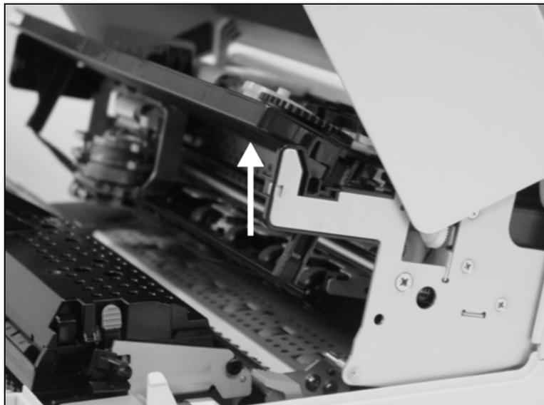
Raise the front end of the ribbon cassette on both sides. Take the ribbon cassette out of the printer.
