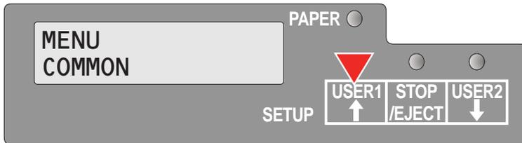
The **USER1 key** is used to go to the next parameter group or next parameter on the same menu level (symbolized by an arrow pointing upwards).
