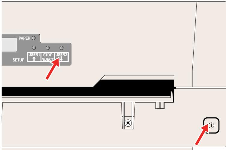
Powering on the printer whilst holding the **USER2** key, and subsequently loading paper on instructions from the LCD panel will allow you to make a status print. This is a print of all the parameter settings. Keep the USER2 key pressed until the message **Print StatusPage Load Paper** appears on the LCD display.
