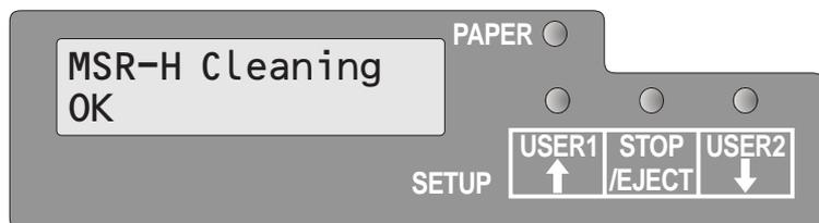
After finishing the cleaning process the LCD displays the Message **MSR-H Cleaning OK**. You can repeat the cleaning routine by pressing the STOP/EJECT key.
