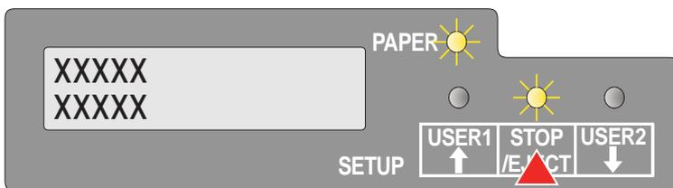
When the Ready and Paper indicators blink, an error has occurred. Annotate the displayed message in the LCD display. By pressing the **STOP/EJECT** key, paper will be ejected if loaded.
