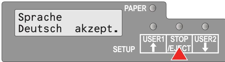
Press the **STOP/EJECT** key to confirm the selection.
