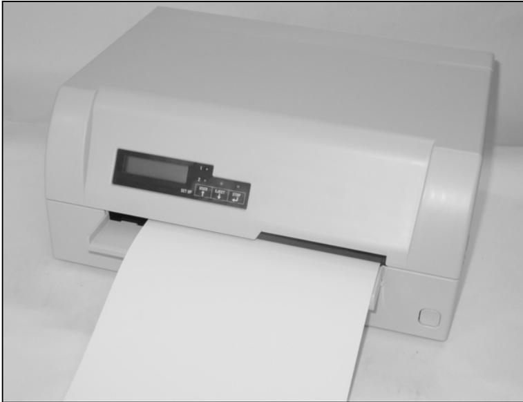
Insert the document in such a way that the right paper edge is positioned inside the area between the left side of the symbol and the right edge of the document support, so that the document alignment can grasp it securely. This is especially important for documents that are narrower than a A4 sheet.
