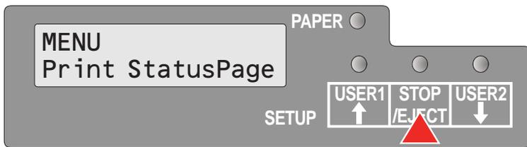
Press the **STOP/EJECT** key.
