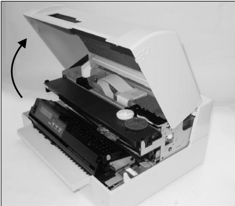
Open the top cover by grasping it at the right and left-hand sides and swing upward until it clicks into position.
