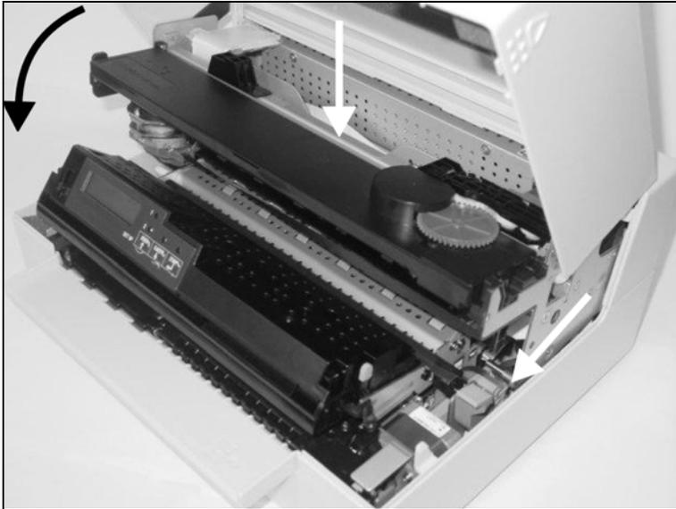
Close the main frame by pressing the colored section in the middle of the frame as shown and ensure both left and right hand sides of the frames are fully latched.
