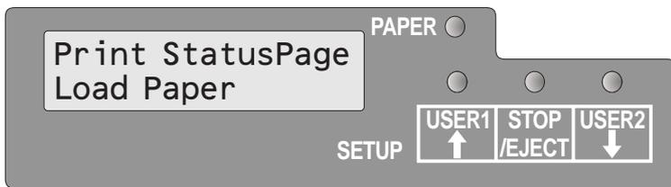
Insert the paper in the printer. The LCD displays **Print StatusPage Printing...** and the status page is printed.
