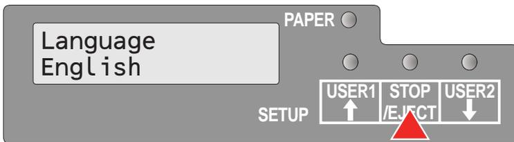
Press the **STOP/EJECT** key. An asterisk appears in the display.
