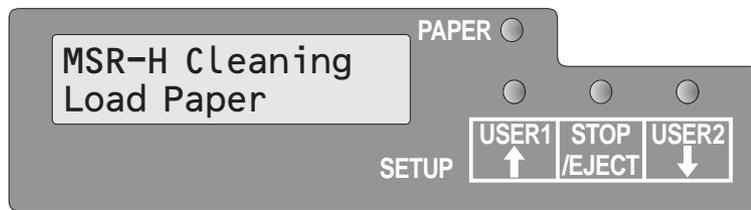
The message **MSR-H Cleaning Load paper** appears on the LCD display.
