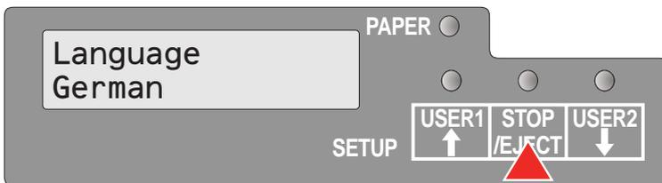
Press the **STOP/EJECT** key.
