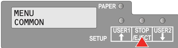
Press the **STOP/EJECT** key.
