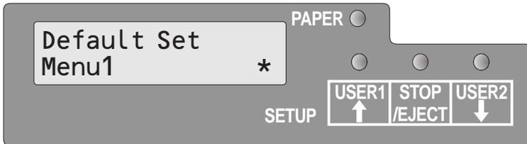
If pressed when a changeable parameter item is on the display, an asterisk appears on the display; you can now change this item now by pressing the **USER1** or the **USER2** key.
