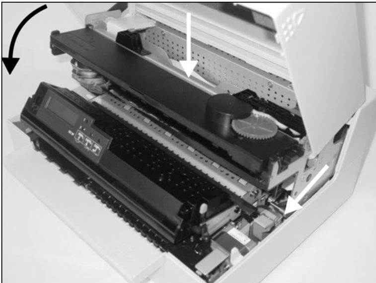
Close the main frame by pressing the colored section in the middle of the frame as shown by the white arrow and ensure both left and right hand sides of the frames are fully latched.
