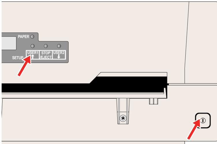
Powering on the printer whilst holding the **USER1 key** will allow you to enter menu mode. Keep the USER key pressed until the message **MENU USER** appears on the LCD display.
