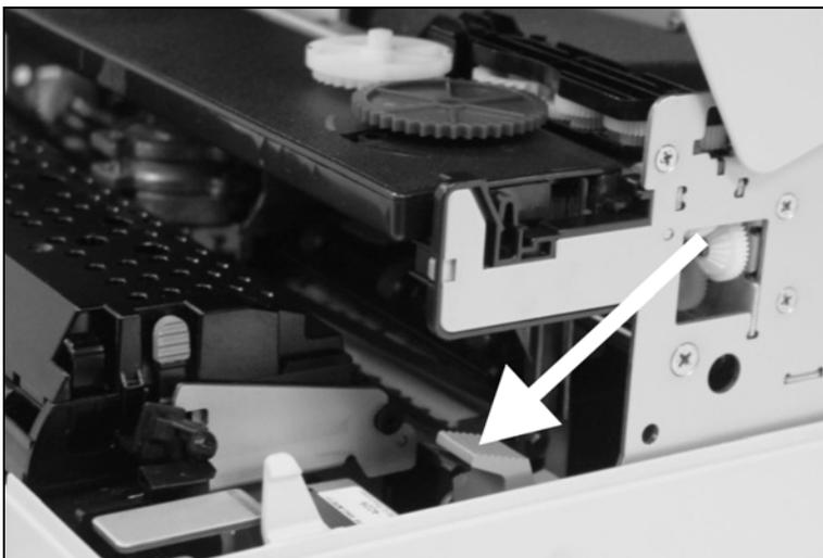
Press the green release lever in the printing mechanism. This will swing the printing mechanism backwards.
