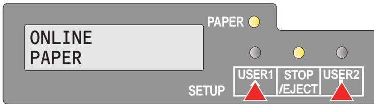
The **USER1** and **USER2** keys are by default inactive. They must be activated via an application. The functionality of the keys then depend on the selected emulation and the sequences sent to the printer.
