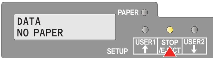
When the printer is online and the Paper indicator is off and there is data in the printer buffer, the LCD displays **DATA/NO PAPER**. You can switch the printer from online to offline by pressing the **STOP/EJECT** key.
