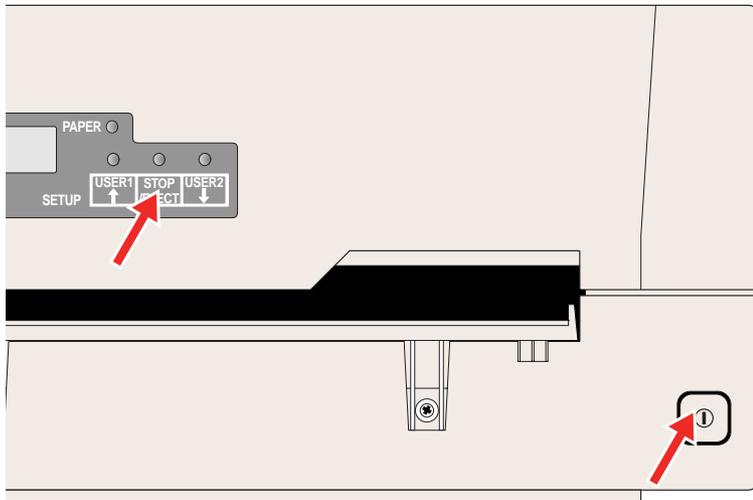
Powering on the printer whilst holding the **STOP/EJECT** key will activate “Hex Dump” mode. Keep the STOP pressed until the message **Hex Dump NO PAPER** appears on the LCD display.
