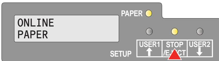
If paper is loaded when the printer is online (Ready and Paper indicator lit), by pressing the **STOP/EJECT** key, the document will be ejected, the LCD displays **REMOVE PAPER**. The printer remains online.
