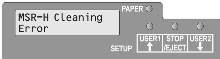
If an error occurs during the cleaning process, the LCD displays the message **MSR-H Cleaning Error** after the cleaning action has ended.
