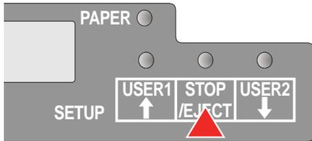
Press **STOP/EJECT** key to save a parameter value. In the second line of the LCD display the message **Accepted** appears. Press **STOP/EJECT** key again to confirm the setting.
