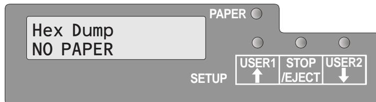
Insert a sheet of paper. The sheet is drawn in. Send the test file from your PC to the printer.
