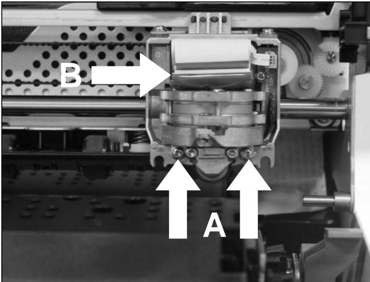
Remove the two outside located screws **A** from the print head.
