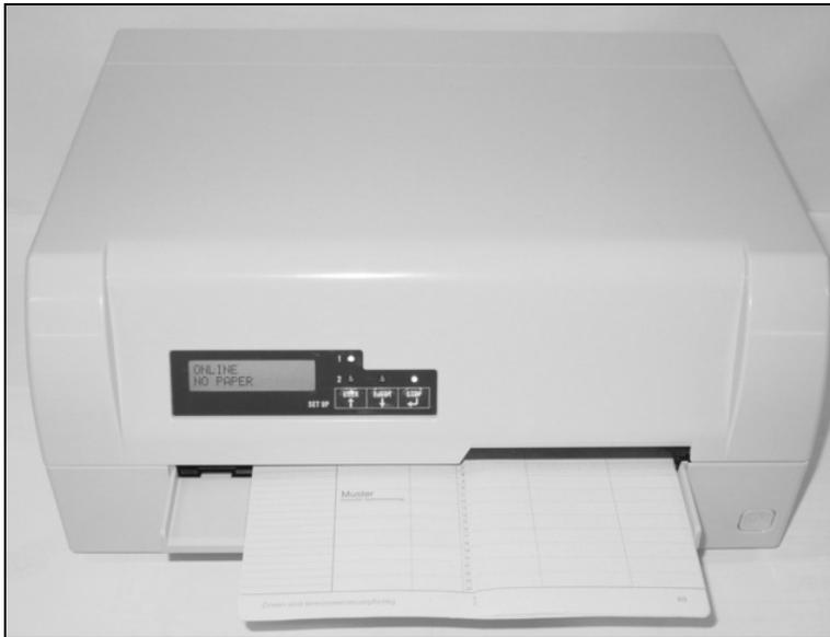
After the passbook is printed, it should be automatically ejected from the printer and released for removal. If the passbook has not successfully ejected from the printer, press the **STOP** key to take the printer to STOP (Offline) mode: press the **STOP** key again to eject the passbook.
