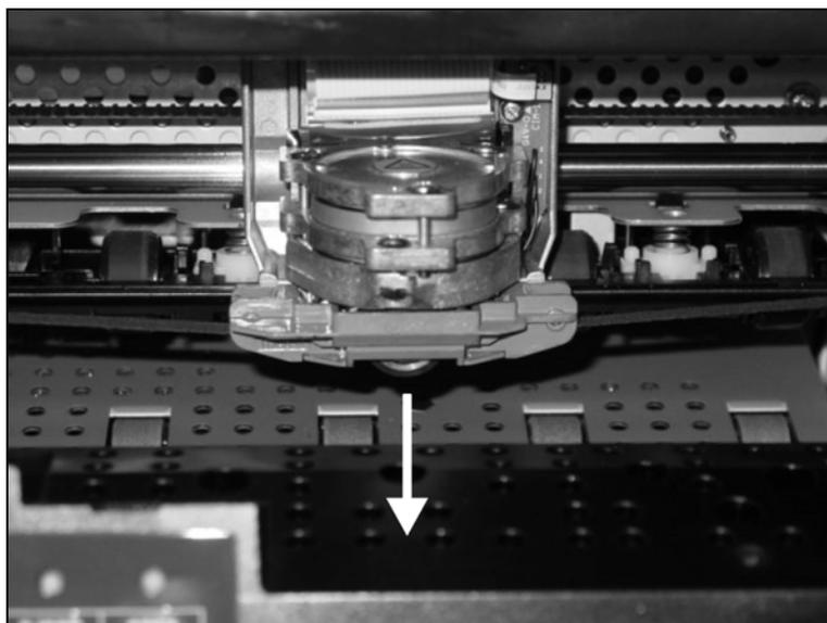
Move the print head to center of the carriage to allow enough room to remove the ribbon guide from the print head.
