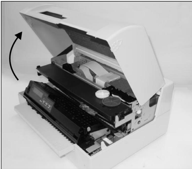
Open the cover by grasping it at the right and left-hand side and swing it upwards until it clicks into position.
