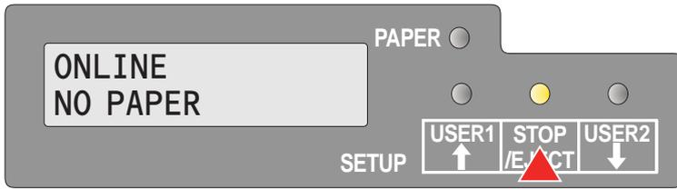
With the Ready indicator lit, the printer is ready to receive data from the host. You can switch the printer from online to offline by pressing the **STOP/EJECT** key.
