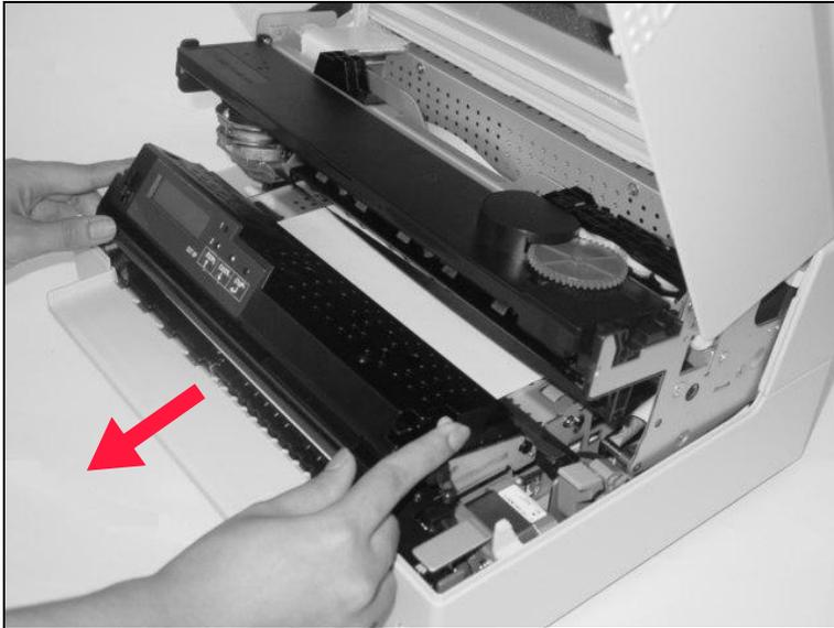
Press the two green release levers on both sides of the panel and lift the panel up. Then remove the jammed paper by pulling it in direction of the arrow out of the printer.
