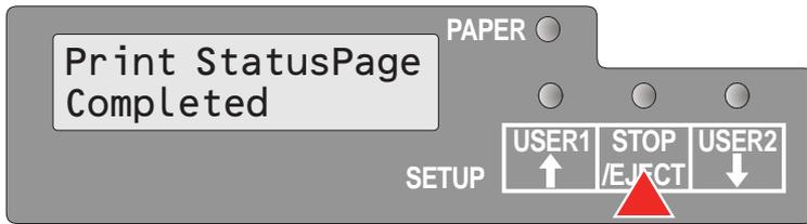
When the test printout is aborted or completed, LCD will display **Print StatusPage Completed**.
