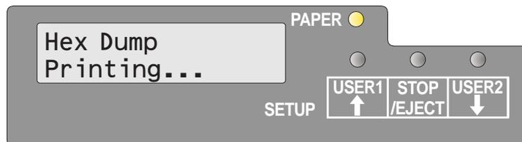
The message **Hex Dump Printing...** is displayed and data is printed. **USER1** and **USER2** keys are invalid during printing.
