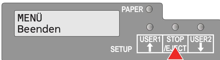
Press the **STOP/EJECT** key. Menu mode is terminated and the printer initializes.
