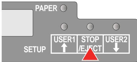
Press the **STOP/EJECT** key to enter to the Parameter select mode. The LCD displays the respective parameter and MENU.
