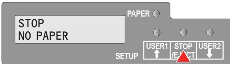
When the Ready indicator is not lit, the printer is Offline and will not receive data. Press the **STOP/EJECT** key to switch the printer Online. Alternatively if paper is still in the printer when in the Off-lline condition, the paper will be ejected.
