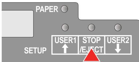
Press the **STOP/EJECT** key to enter the MENU setting mode.
