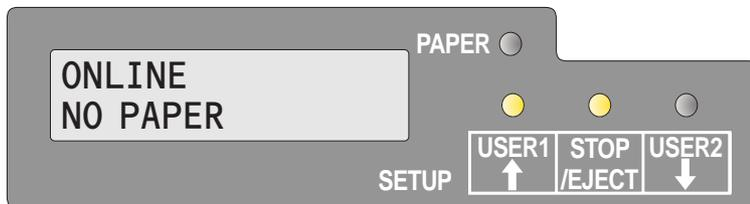
When initialization is completed, the Ready indicator and the USER1 indicator light up. The message **ONLINE NO PAPER** appears on the LCD. The printer is in the online status and ready to accept data from the system. You can now insert a document or passbook.
