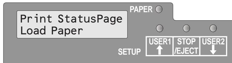
The LCD displays **Print StatusPage Load Paper**. Release the **USER2** key.
