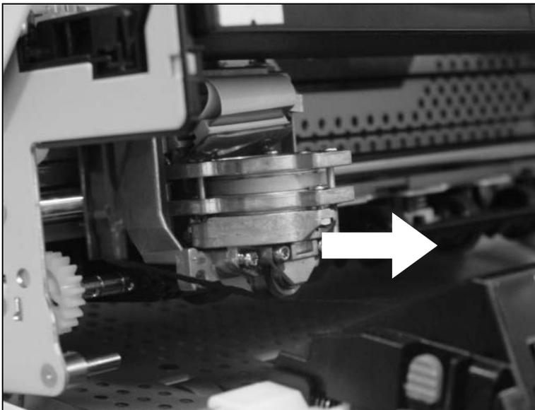
Now remove the print head from its mounting by easing it forward.
