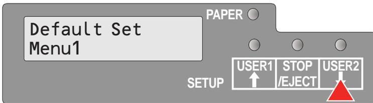
Press the **USER2** key several times, until in the LCD display appears:
