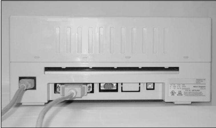
Make sure that the printer and the computer are switched off and connect the data cable between the printer and the computer. This example shows a 36-pin centronics parallel cable.
