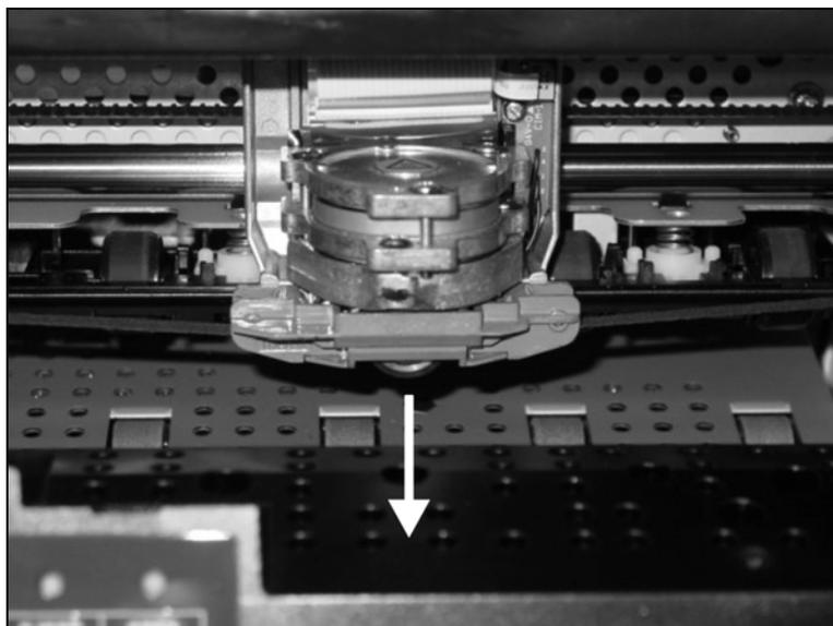
Remove the colored ribbon guide from the print head by pulling it downwards.
