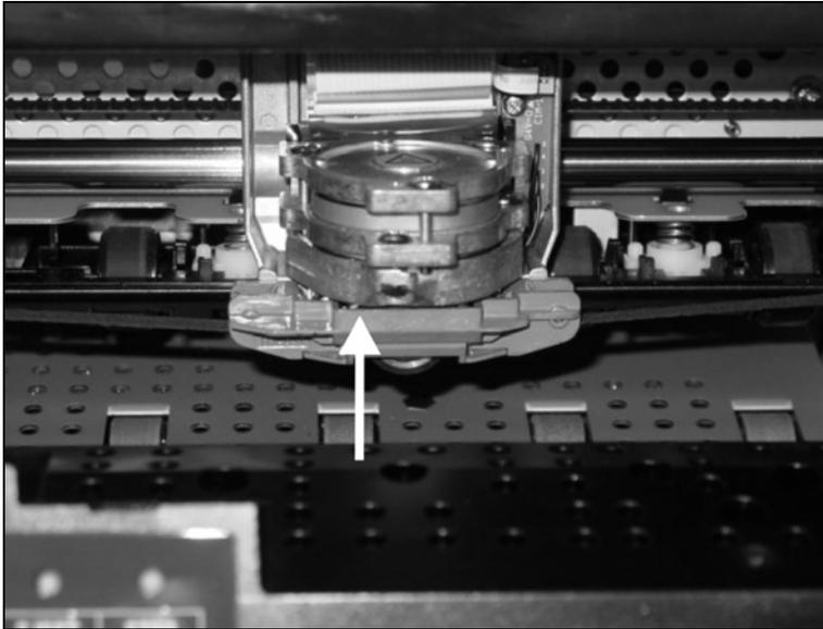
Pull the ribbon guide under the print head. Tighten the ribbon by turning the tension gear in the direction of the arrow (see image below).
