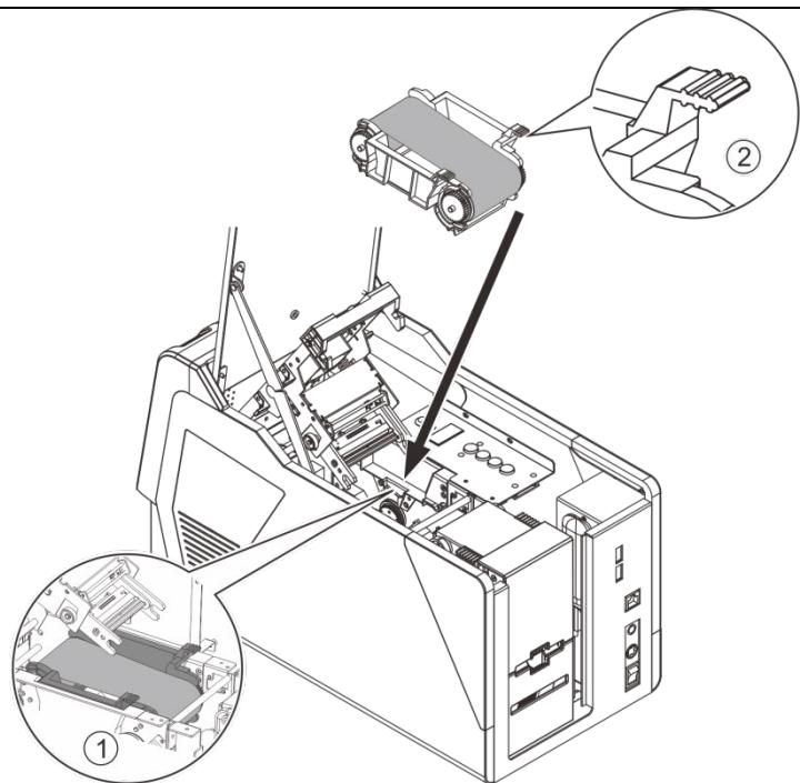
(1) When the Ribbon roller is mounted to the cartridge base, push it down to the bottom with a little force.
