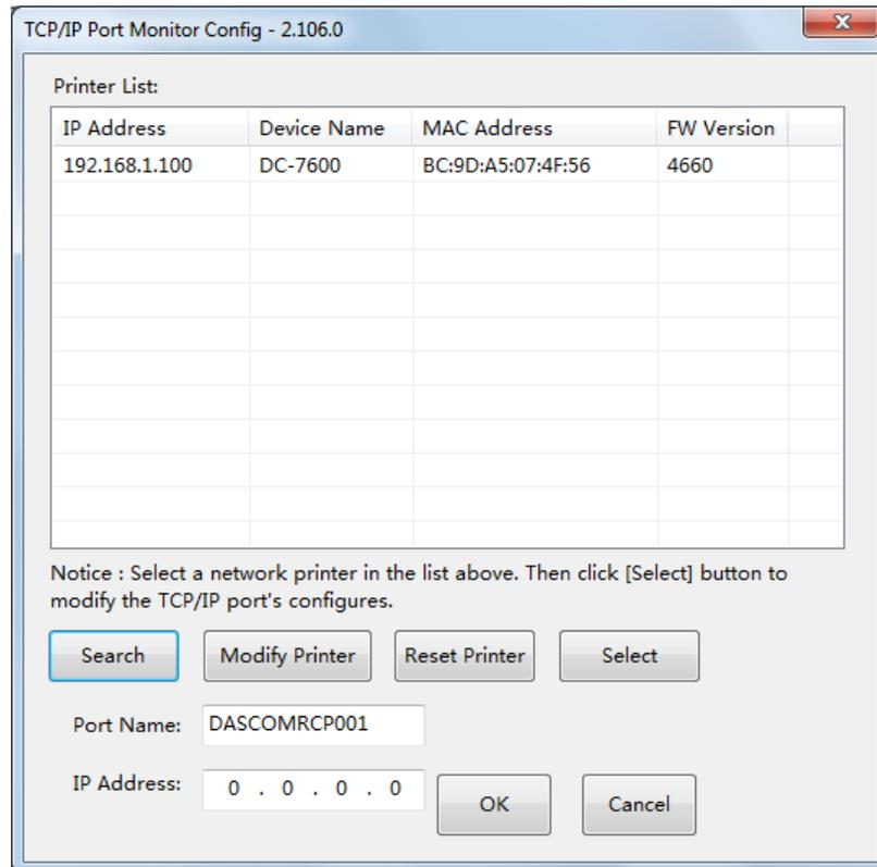
(4) You can modify the Printer name, IP address acquisition mode, IP address, Subnet mask. Click the “OK” when you finish.
