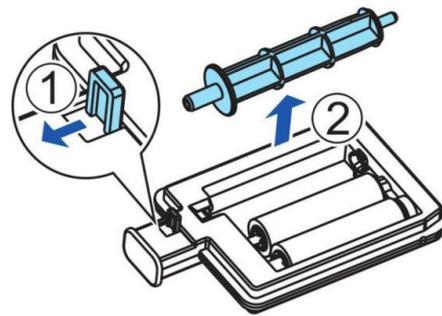
Sleeve a new **cleaning roller** into the **spindle**.
