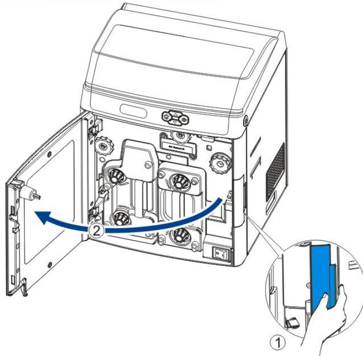
Directly pull out the **cleaning cartridge** to release it from lock position.
