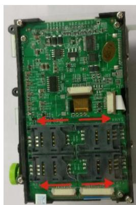
Put the card into the corresponding position of the slot, close the slot cover, then push the slot cover. When you hear a click, the card is installed properly.
