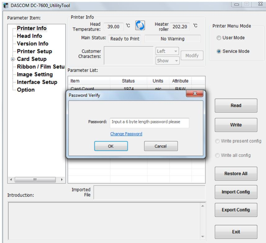
In service mode, user can modify the print position, print density, system settings, print head, option state and configuration. Please don't random change them, it may lead to poor printing effect.
