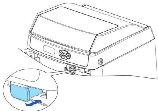
Pull the **lock**① to release the **spindle**②.
