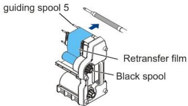
As shown in the right diagram, push in the retransfer film cartridge to the far end until a "click" is heard to indicate correct insertion.
