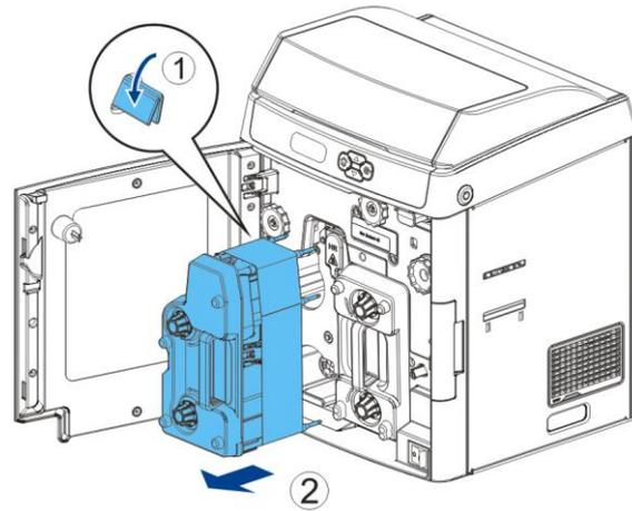
To load new retransfer film onto the cartridge, engage the **green spool** ① of the retransfer film to the feeding hub of the cartridge.
