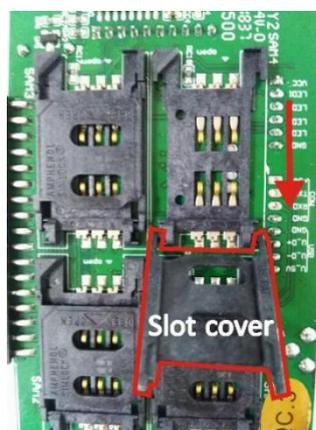
Put the card into the corresponding position of the card slot, close the card slot cover, then push the card slot cover in the direction indicated by the arrow. When you hear a click, the card is installed properly.
